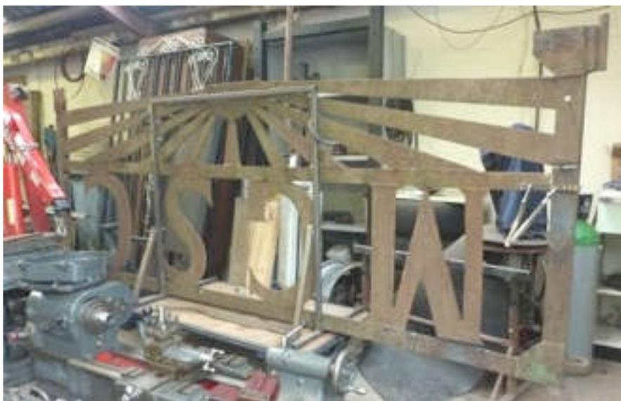
The lowest bar running across the whole width of the gate had been buried in the ground for many years, so that has mostly rusted away. Fortunately, Andrew has found another piece to weld in place, of an age which will match the other sections of the gate. This is the piece which will be welded under the sun burst.
